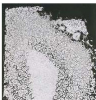
HASTELLOY® X alloy Average Metal Affected = > 22 Mils (560 μm)/Side
