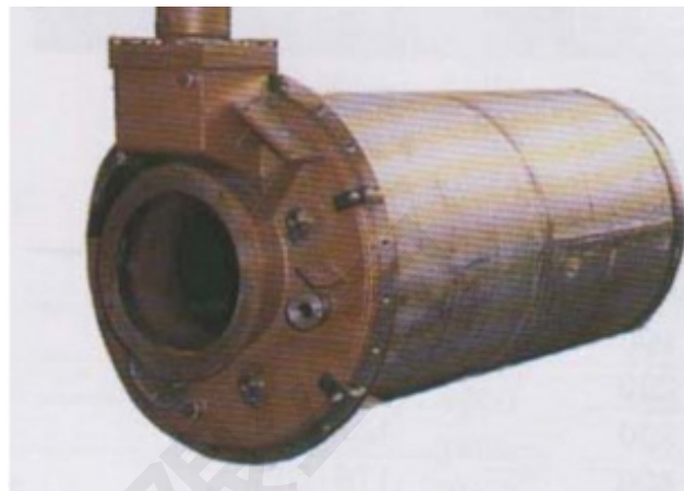
556 alloy vacuum carburizing furnace retort.
