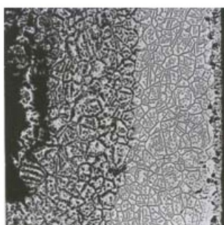
INCONEL alloy 601 Average Metal Affected = > 22 Mils (560 μm)/Side
